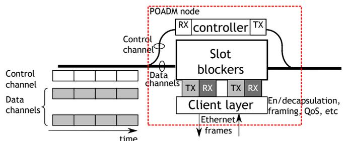
Fig. 1. Optical slot switching POADM node description.
