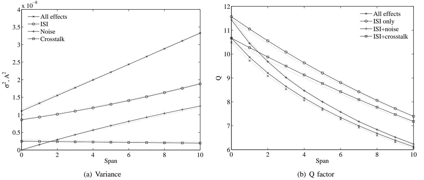
Fig. 3. Details of the impact of each impairment on a 10 GHz dispersion-compensated system: noise, ISI, crosstalk.
