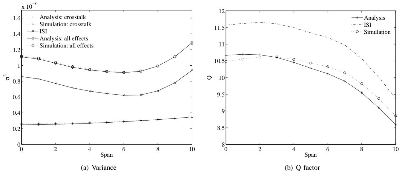
Fig. 4. Details of the impact of ISI and crosstalk on a 2.5 Gbps system.
