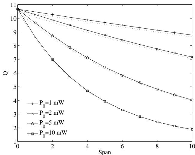
Fig. 6. Impact of the main signal peak power.
