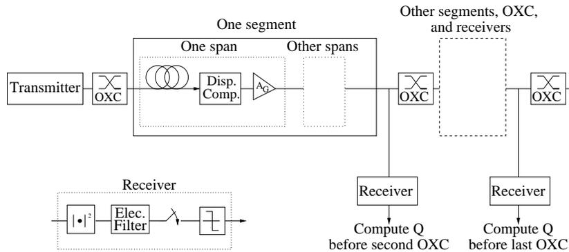
Fig. 2. **Simulated network.** Each OXC adds a crosstalk component to the input signals.
