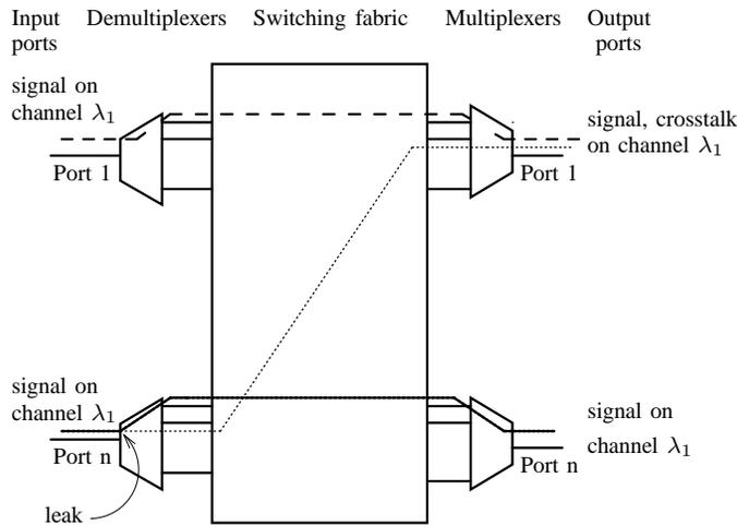
Fig. 1. **Source of in-band crosstalk.** Due to filter imperfection in the OXC, a small amount of the input signal on channel  $\lambda_1$  on the  $n^{\text{th}}$  input port is allowed in the switching fabric via the input reserved for channel  $\lambda_2$ .
